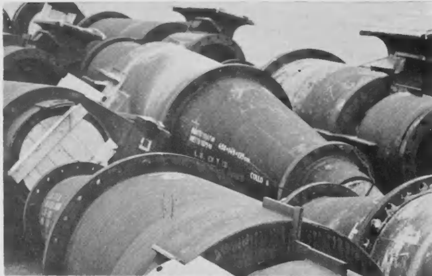
NEW CYCLONES will be installed in the PCAR Cat Cracker next spring. The cyclones will be hung upright in the reactor to separate the catalyst from the vapors. Dust pots are secured below them, with diplegs extending downward into the catalytic agent.
